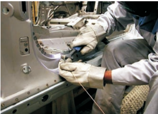
Figure 22: Manual plasma brazing on the door sill of a BMW car body
