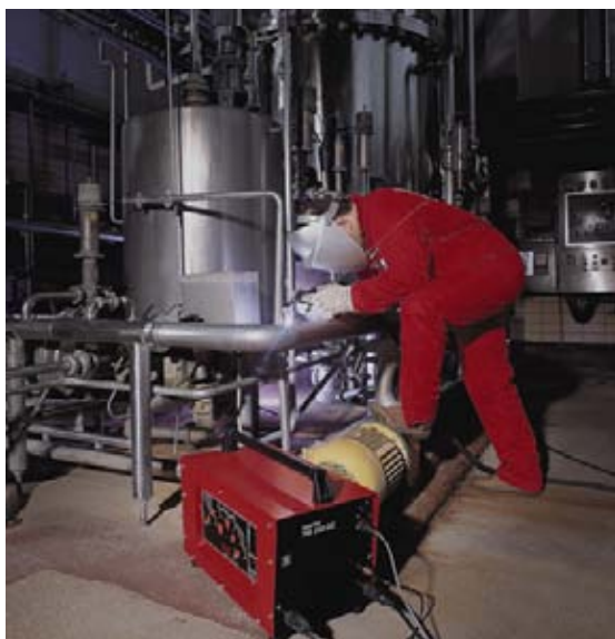
Figure 24 TIG 230 DC, TIG welding in the food industry
