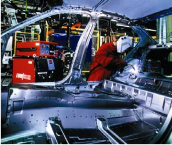
Figure 41 MIG brazing in assembly vehicle bodywork
