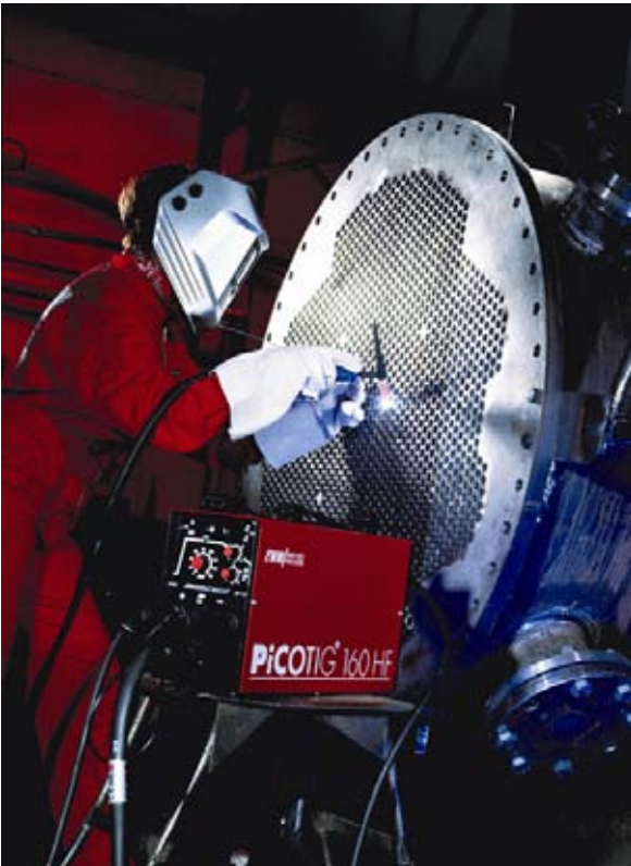
Figure 32 TIG welding used to weld pipes into pipe bends
