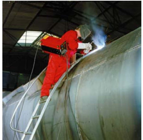
Figure 21 Use of MMA welding in container construction
