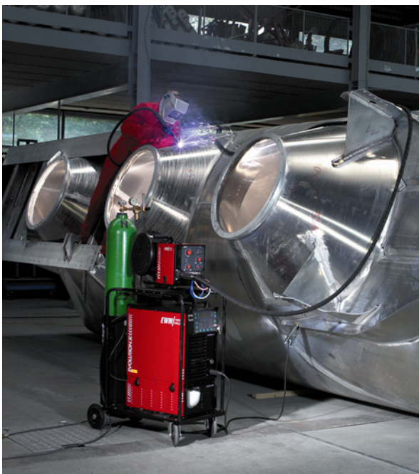
Figure 39 MIG aluminium welding in vehicle construction
