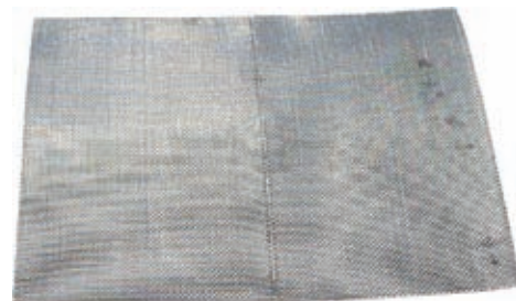
Figure 20: Longitudinal seam on protective grids for chemical ovens
