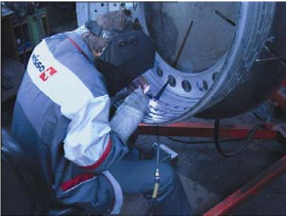
Figure 31 TIG welding in the repair of drive unit components
